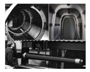
Figure 3. Internally stiffened thermoplastic composite tail boom.
