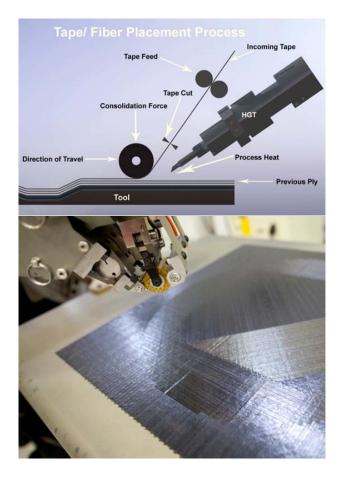
Figure 1. Schematic and photo of the automated fiber placement process.
