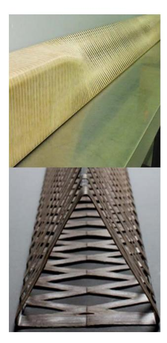
Figure 4. Fiberglass composite beams for a ceiling support concept.
