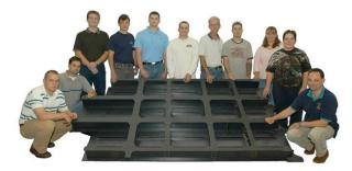
Figure 2. Carbon fiber composite sub-floor for the H-60 Blackhawk helicopter.
